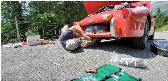
Finally, the exhaust system cooled enough to pick it up and we shoved it into the main exhaust pipe under the transmission. Through a complex engineering process, which involved a large rock and my BRAND NEW lead wire wheel hammer, we were able to beat the exhaust system into submission. Once the beating commenced, the rear pipe got close enough to the rear frame tube (under
